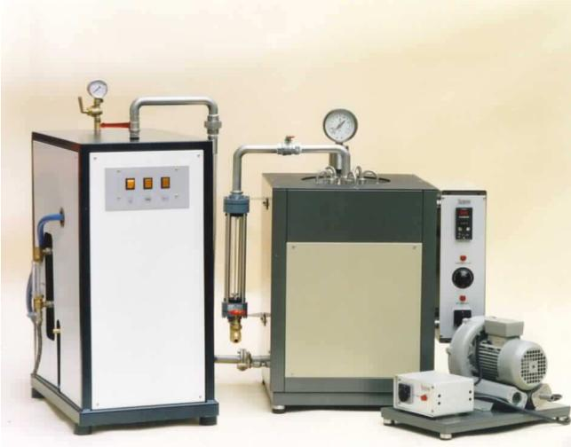
Apparatus (center) with steam generator (left) and air blower
