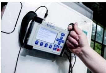
Two powerful rear magnets for instrument positioning on metal surfaces...
