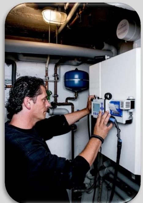
View ecom-D in full, optional equipment: thermal quick printer module, mini gas cooler and NOx sampling tubing
