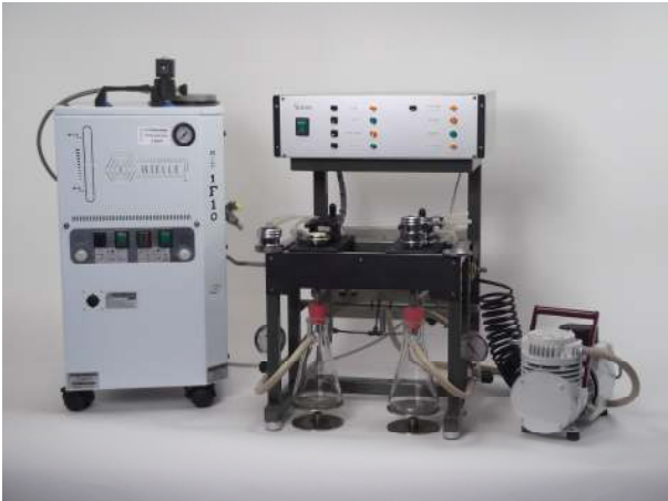
Steam generator, automatic apparatus and vacuum pump
