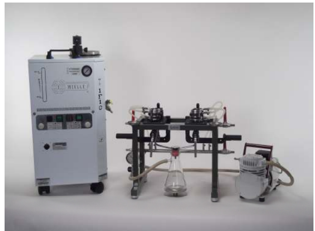
Manual apparatus with steam generator and pump
